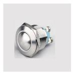
Diameter: Ø 22mm Switch Rating: 5A/250VAC Contact Configuration: 1NO Operation Type: Momentary The Front Shape: Ball The Crust Material: Stainless steel IP Degree: IP67, IK10
