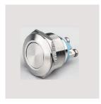
Diameter: Ø 22mm Switch Rating: 5A/250VAC Contact Configuration: 1NO Operation Type: Momentary The Front Shape: Flat
