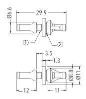
① FANS MOUNTING HOLE Ø4.6±0.2 AND 3.0 ~5.5 THICKNESS. ② SUPPORT MOUNTING HOLE Ø6.5±0.1 AND 1.0~2.0 THICKNESS.
